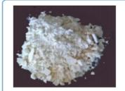
Aragonite, another form of calcium carbonate, has very different characteristics to calcite. When calcium carbonate precipitates as argonite it forms a non-adhering harmless insoluble crystal that is either consumed or carried through the system to the drain.
